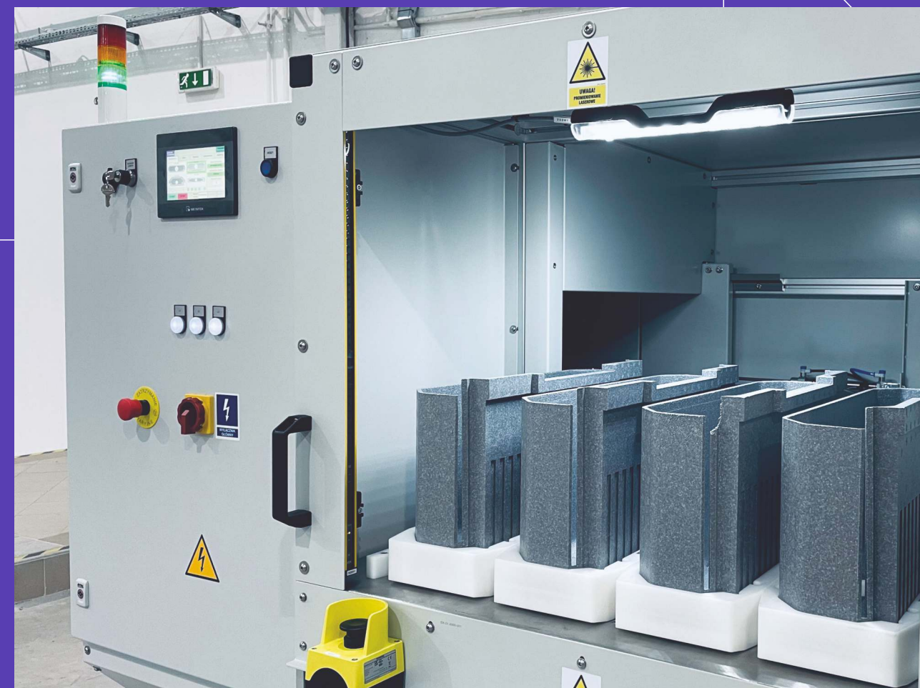
Laser Marking Stations for Insulation Elements in Water Tanks for Concealed Toilet Systems.
