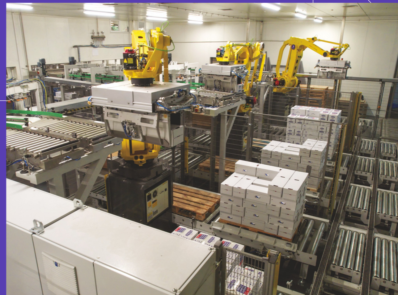
Robotic Palletizing Station for Butter
